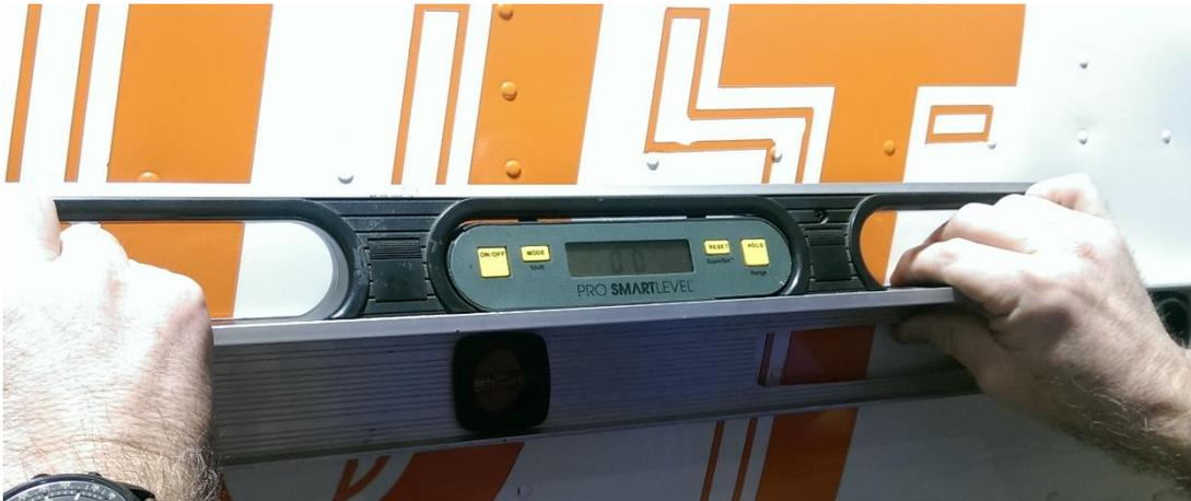
Figure 13: Aircraft water level reference line. The ADS Boom aligned with this reference line; the INS unit has a 0.1° offset from this reference line.
