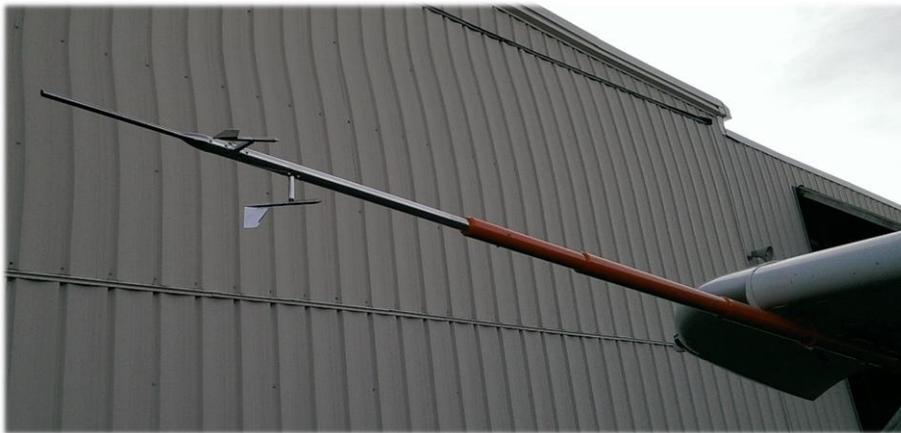
*Figure 1: NACA Air Data Boom Design with Flow Angle Vanes on the UTSI Cessna 210 right wingtip.*
